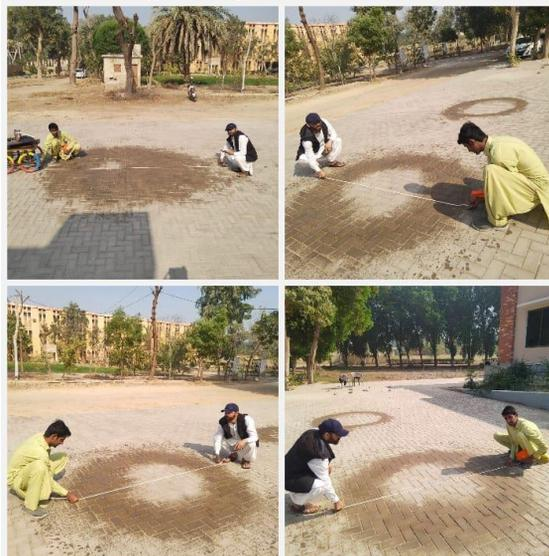
Figure 10. Measuring the discharge, inner and outer area covered
