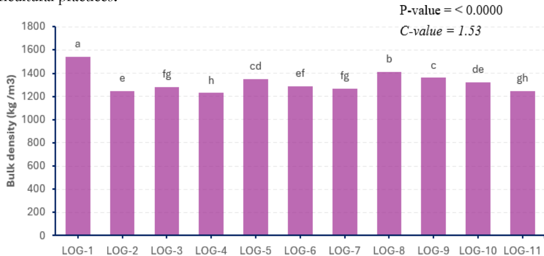
Figure 7. Bulk densities of different logs. Different alphabets (a,b,c,d) among the mean values show significant differences at P < 0.05
