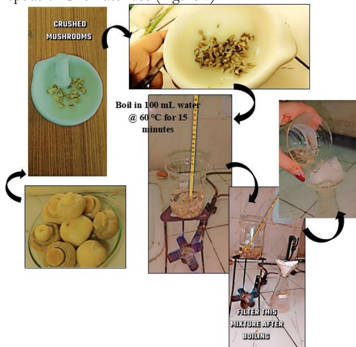
Figure 7. Flow diagram: Preparation of button mushroom extract (ethanolic and aqueous extract)
